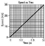
$$a = \frac{\Delta v}{t} = \frac{30. \text{ m/s}}{3.0 \text{ s}} = 10. \text{ m/s}^2$$
