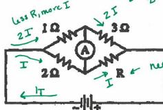
If the ammeter in the circuit above reads zero, what is the resistance R? Keep RATIO of R the same
