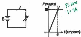
A graph of the power *P* dissipated in the resistor as a function of the current *I* supplied by the battery is also given above. What is the emf of the battery?
