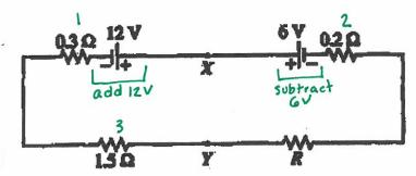
In the circuit above, the emf's and the resistances have the values shown. The current I in the circuit is 2 amperes.
