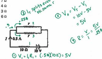
In the circuit shown above, the value of r for which the current I is 0.5 ampere is
