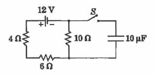
The circuit shown above includes a battery which has zero internal resistance.
