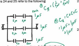
The diagram above shows a system of six/2-microfarad capacitors.
