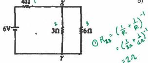
In the circuit shown above, what is the value of the potential difference between points X and Y if the 6-volt battery has no internal resistance?
