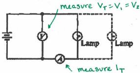
Connecting another lamp in parallel with the first as J R. TIT shown by the dashed lines would
