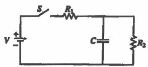
In the circuit shown above, the battery supplies a constant voltage V when the switch S is closed. The value of the capacitance is C, and the value of the resistances are R1 and R2.
