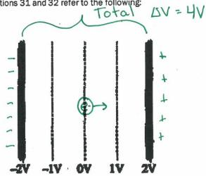
A battery or batteries connected to two parallel plates produce the equipotential lines between the plates shown above.
