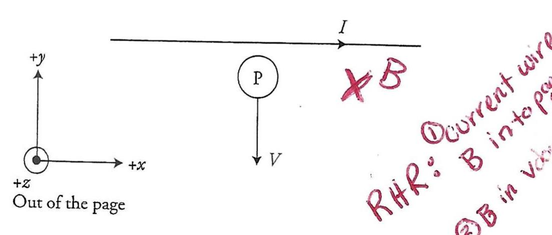
11. A proton with a velocity v is moving directly away from a wire carrying a current I directed to the right in the +x direction as shown in the figure. The proton will experience a force in which direction?
