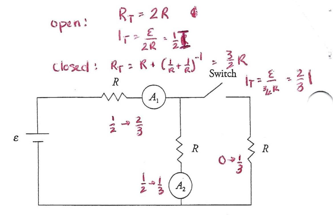
6. The circuit shown has a battery of emf  $\varepsilon$ ; three identical resistors, R; two ammeters,  $A_1$  and  $A_2$ ; and a switch that is initially in the open position as shown in the figure. When the switch is closed, what happens to the current reading in the two ammeters?
