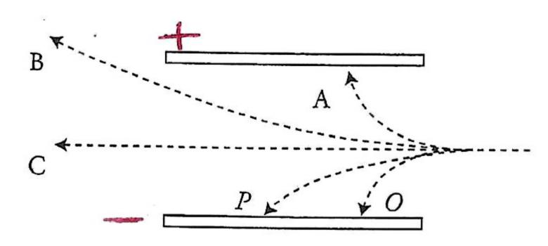
1. A beam of various particles is launched into the space between two oppositely charged parallel plates as shown in the figure. It is known that the particles are all traveling at the same initial velocity as they enter the region, and that particle P is a proton. What else can be inferred?
