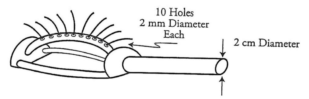
20. A 2-cm diameter hose leads to a lawn sprinkler with ten 2-mm exit holes as shown in the figure. The velocity of the water in the hose is  $v_1$ . What is the velocity of the water exiting the holes?
