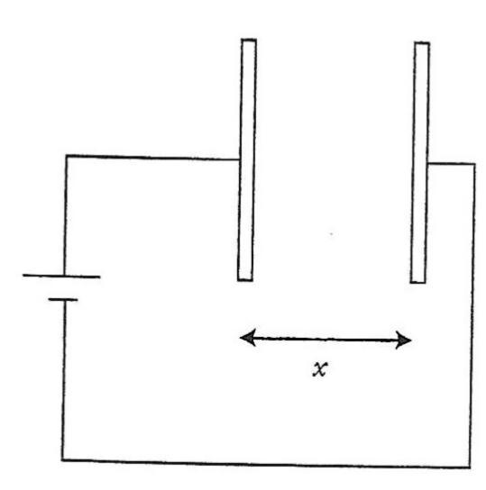
10. A capacitor with movable parallel plates is connected to a battery. The plates of the capacitor are originally a distance x apart as shown in the figure. With the battery still connected, what happens to the energy stored in the capacitor and the electric field between the capacitor plates, if the plates are moved to a new distance x/2?
