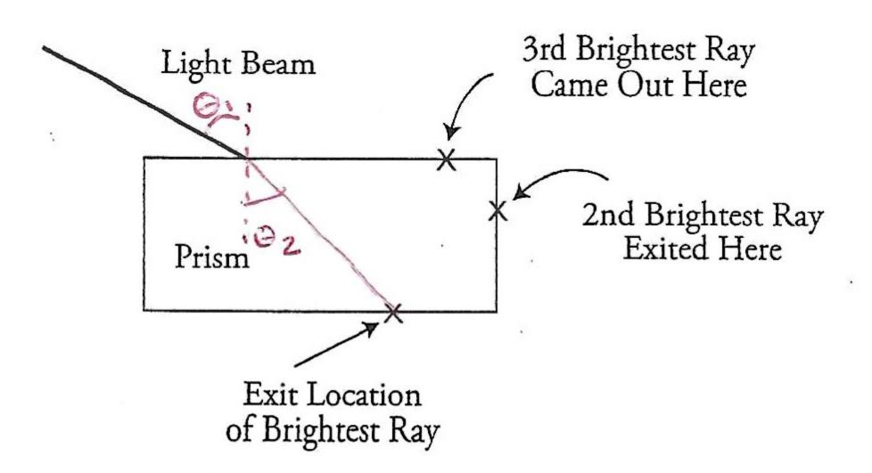
16. Your lab group has been asked to determine the index of refraction of a plastic rectangular prism. Your partner places the prism on a sheet of paper, traces its shape, shines a beam of light through the prism, and traces the incoming ray. The light exits the prism at multiple locations. Your partner marks the exit locations of the three brightest rays on the side of the prism as shown in the figure. Is this enough information to determine the index of refraction of the prism and why?
