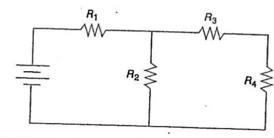
47. Which placement of voltmeters will allow for determination of the voltage across resistor R2 in the circuit diagrammed in the preceding figure? Choose two answers,
