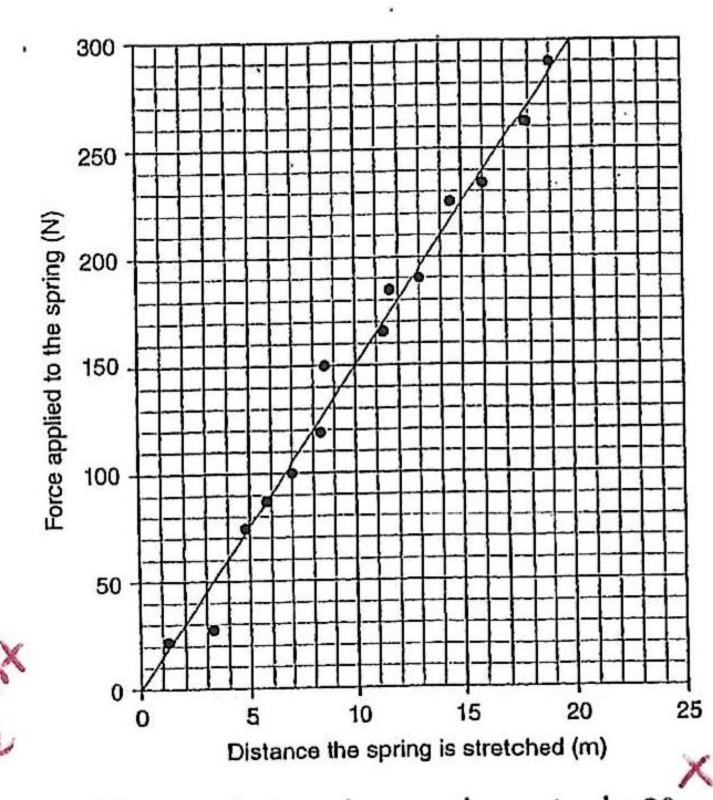
27. A force probe is used to stretch a spring by 20 cm. The graph of the force as a function of distance shown in the preceding figure is produced and used to determine the amount of work done in stretching the spring 20 cm. The experimenter reports the result as 3,000 J. Which of the following is a reasonable estimate of the experimental uncertainty on this measurement? 1000
